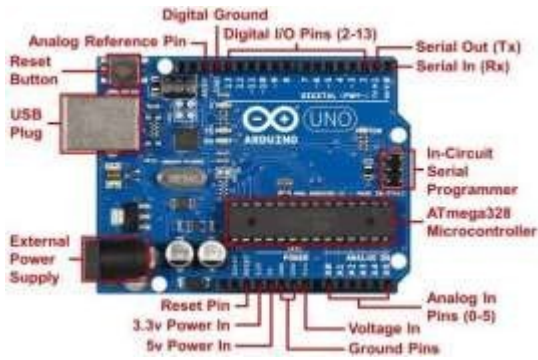
Fig. 3. Arduino Uno R3 with pin-outs.
